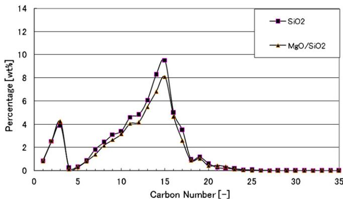
**Fig. 4.** Carbon number distribution of SiO<sub>2</sub> based catalyst. Oil feed rate: 15 ml/h, catalyst: 50 ml, LHSV: 0.3 h<sup>-1</sup>, temperature: 703 K, pressure: 0.1 MPa, carrier gas (He): 50 ml/min, –■–: SiO<sub>2</sub>, –▲–: MgO/SiO<sub>2</sub>.
