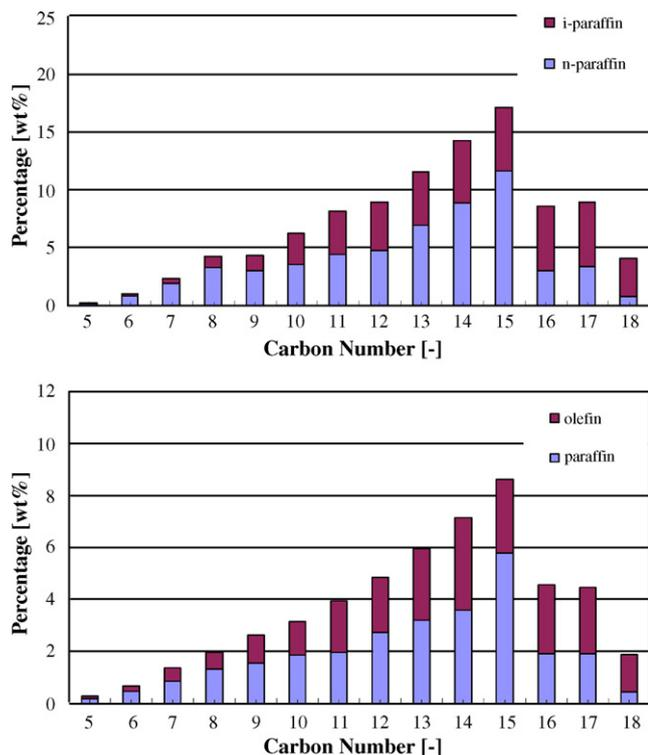
**Fig. 5.** Chemical structure of product hydrocarbons (the same oil with Fig. 3). Oil feed rate: 15 ml/h, catalyst: 50 ml, LHSV: 0.3 h<sup>-1</sup>, temperature: 703 K, pressure: 0.1 MPa, carrier gas (He): 50 ml/min, ■: i-paraffin, ■: n-paraffin, ■: paraffin, ■: olefin.
