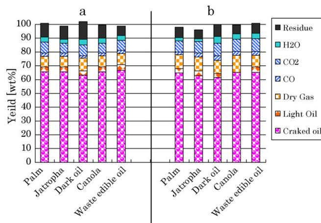
**Fig. 6.** Material balance of various vegetable oils. (a) MgO–SiO<sub>2</sub> catalyst, (b) MgO–active carbon catalyst. Oil feed rate: 15 ml/h, catalyst: 50 ml, LHSV: 0.3 h<sup>-1</sup>, temperature: 703 K, pressure: 0.1 MPa, carrier gas (He): 50 ml/min, ■: residue, ■: H<sub>2</sub>O, ■: CO<sub>2</sub>, ■: CO, ■: dry gas, ■: light oil, ■: cracked oil.
