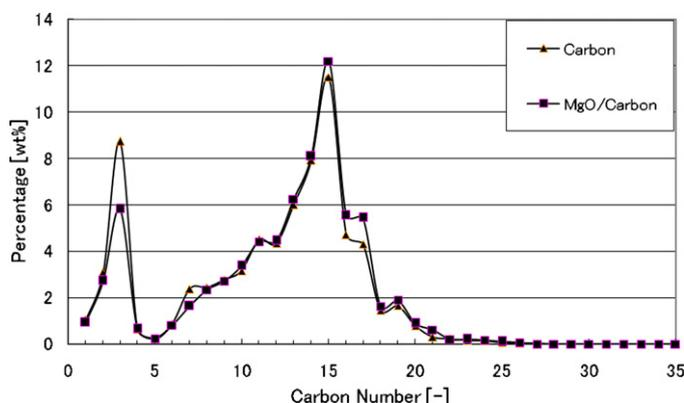
**Fig. 3.** Carbon number distribution of carbon based catalyst. Oil feed rate: 15 ml/h, catalyst: 50 ml, LHSV: 0.3 h<sup>-1</sup>, temperature: 703 K, pressure: 0.1 MPa, carrier gas (He): 50 ml/min, –▲–: carbon, –■–: MgO/carbon.
