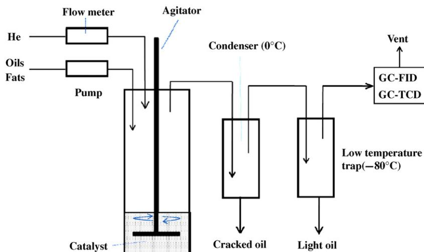
Fig. 1. Reaction apparatus for the catalytic cracking.
